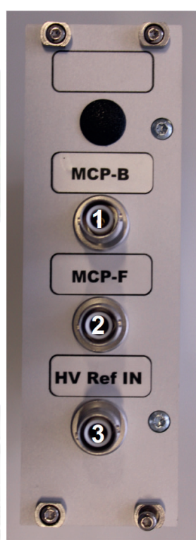
Figure 2: Layout of the 19" HVPS Detector Supply R020.
